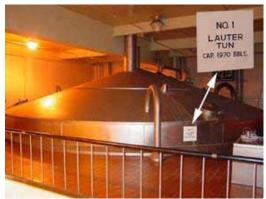
The brew house at the City Brewery is massive, and I have included a couple photos for scale. The lauter tun feeds four large boilers, and holds 1970 barrels (over 60,000 gallons). Their bottling lines have the capability of producing over 70,000,000 cases a year.
