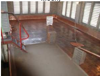
The coolship in the old brewery, where the wort was cooled from boiling to about 140°F. It was poured out on that paddle on the right - hot side aeration anyone?
