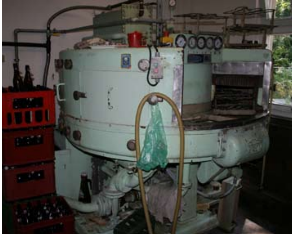
The bottle washer. Looks like a steam line is still attached.
